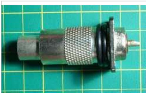
Place the O-ring(s) at the base of the SO-239 barrel and use the PL-259 coupling ring to compress them into a weather-tight seal.
